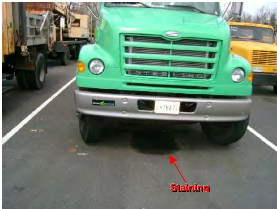
Photograph 26. Central Garage – Staining underneath vehicle indicates a lack of BMP implementation.
