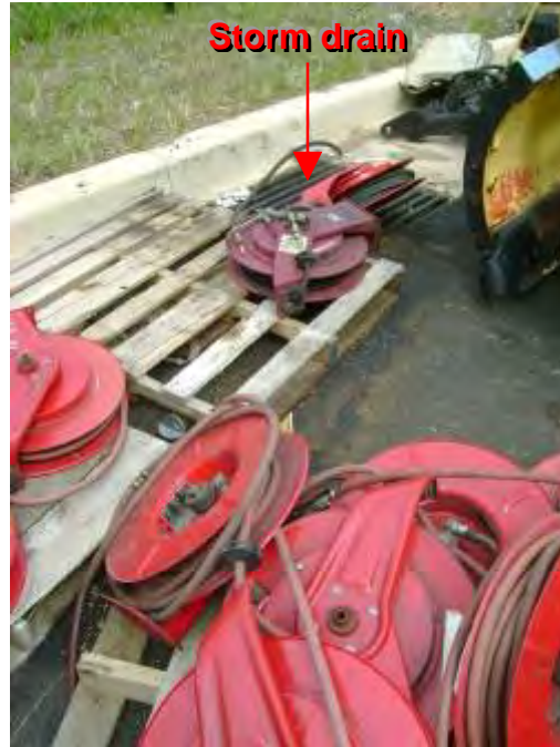
Photograph 17. Central Garage – Close up of used oil hoses near and on top of storm drain (NOTE: Staining around storm drain).
