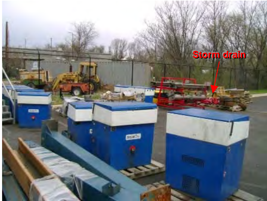
Photograph 19. Central Garage – Parts washers full of parts washing solvent located outdoors and close proximity to storm drain
