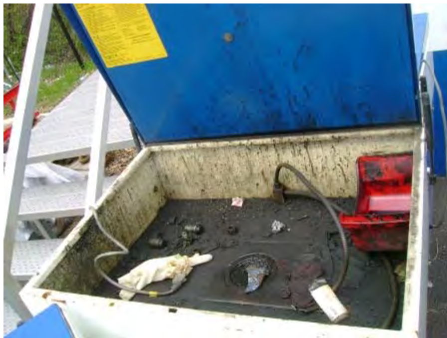
Photograph 20. Central Garage – Example view of the interior portion of the parts washer. (NOTE: Rags and parts still contained within parts washer)
