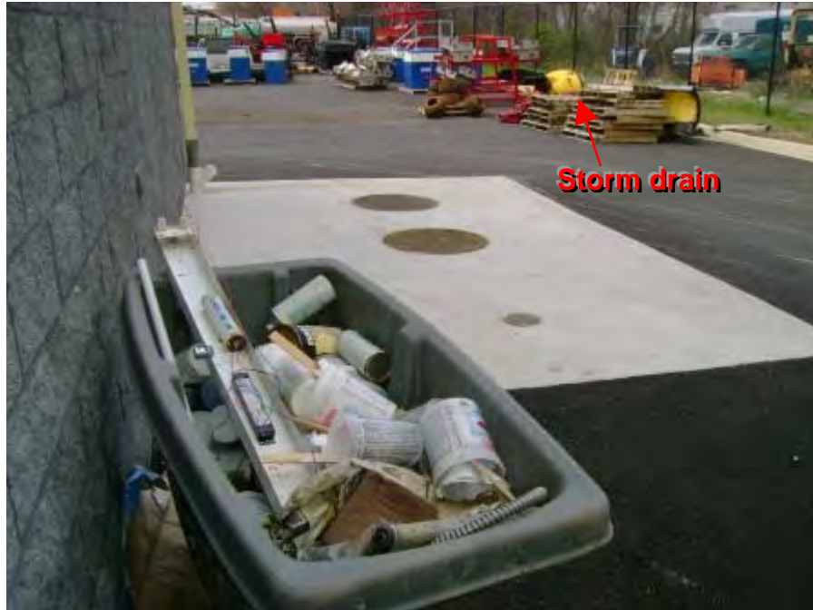
Photograph 21. Central Garage – View of small dumpster containing paint waste and other materials stored in close proximity to storm drain.
