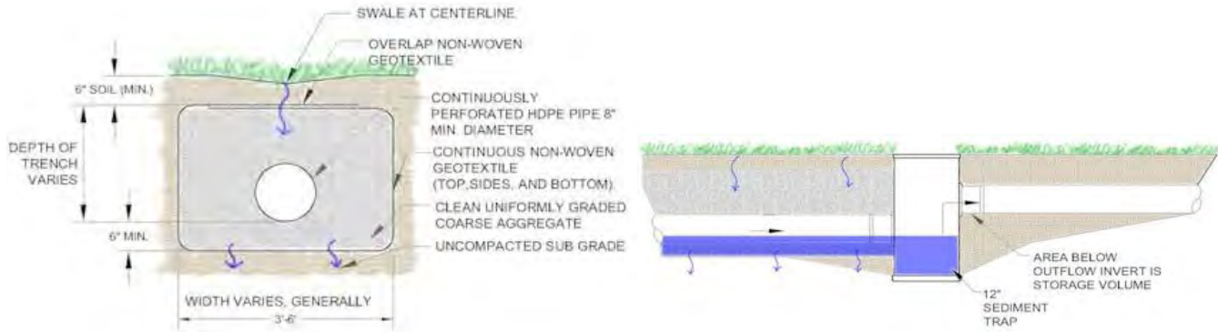
Figure 2: Infiltration Trench Diagram
