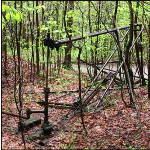
Historic oil wells (Left), piping systems, and storage tanks (Center) can be seen throughout the northern portion of the watershed. These old oil wells can provide a conduit for mine drainage to reach the surface. Discharges BC14 and BC15 severely impact Blacks Creek as can be seen downstream at sampling point 906-42 (Right).
