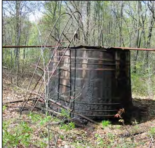
Historic oil wells (Left), piping systems, and storage tanks (Center) can be seen throughout the northern portion of the watershed. These old oil wells can provide a conduit for mine drainage to reach the surface. Discharges BC14 and BC15 impact Blacks Creek as can be seen downstream at sampling point 906-42 (Right).
