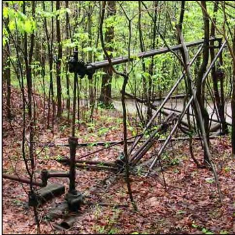
Historic oil wells (Left), piping systems, and storage tanks (Center) can be seen throughout the northern portion of the watershed. These old oil wells can provide a conduit for mine drainage to reach the surface. Discharges BC14 and BC15 impact Blacks Creek as can be seen downstream at sampling point 906-42 (Right).
