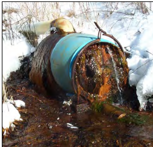
Existing treatment pond TB1 (Left) receives mine discharges MC1, MC2, and MC3 which emanate from the "McIntire" site. The effluent of TB1 (Right) used to be the headwaters of tributary #15. The natural formation of iron minerals at low pH, plugging old piping (Center), has been incorporated into the passive system design.
