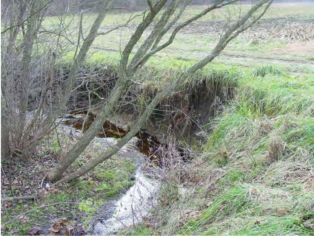
Figure 8 - Typical incised bank on the outside of a turn in the stream due to high flow bank scour.
