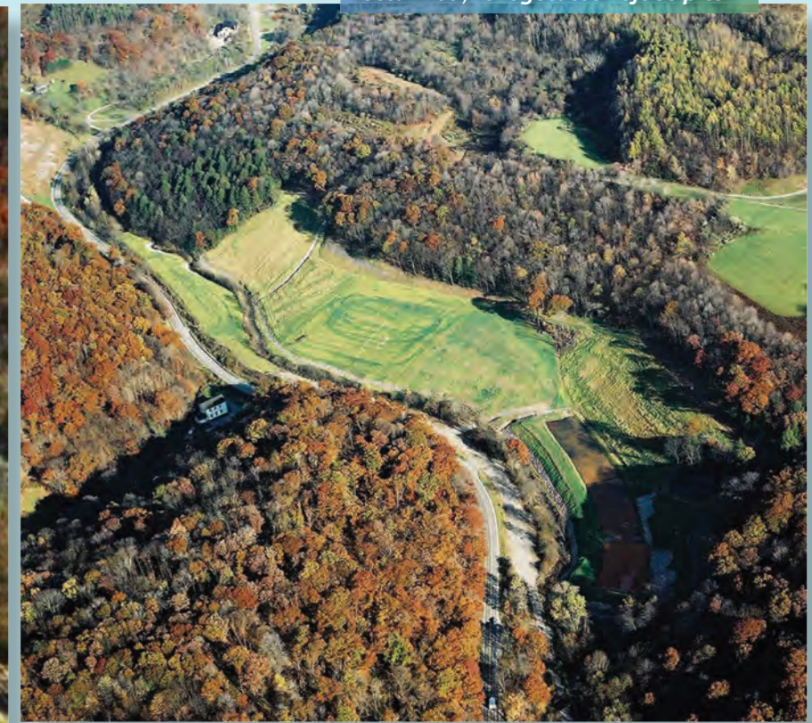
Completed project showing reclaimed, revegetated refuse pile.
