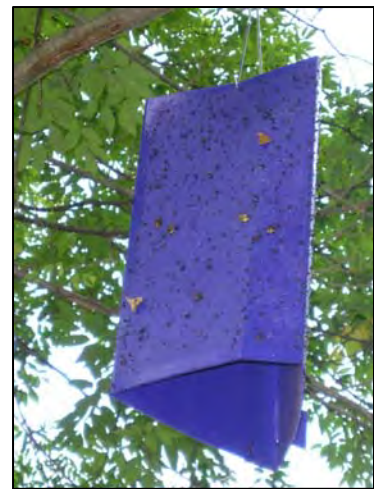
A surveillance trap used to detect the presence of emerald ash borer and other insect populations
