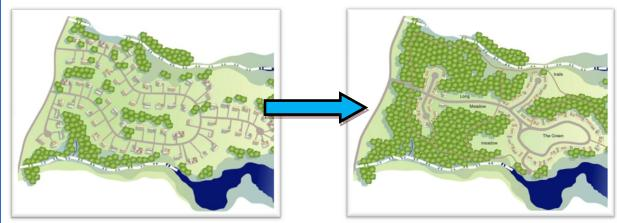
Clustering uses and building on the smallest area possible (above right) generates significantly less stormwater quantity and quality challenges than conventional development (above left).
