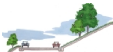
Current cross-section of Overlook Drive and slope adjacent to The Oval. Parking is continuous along the street, access up the slope is limited and maintaining the slope is difficult.
