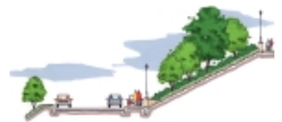
Proposed cross-section showing a new pedestrian walk along Overlook Drive, with new lighting and access steps up to The Oval. Parking should be organized around curb bump-outs at each of the steps. In this way, cars will not block visual or physical access to the steps.
