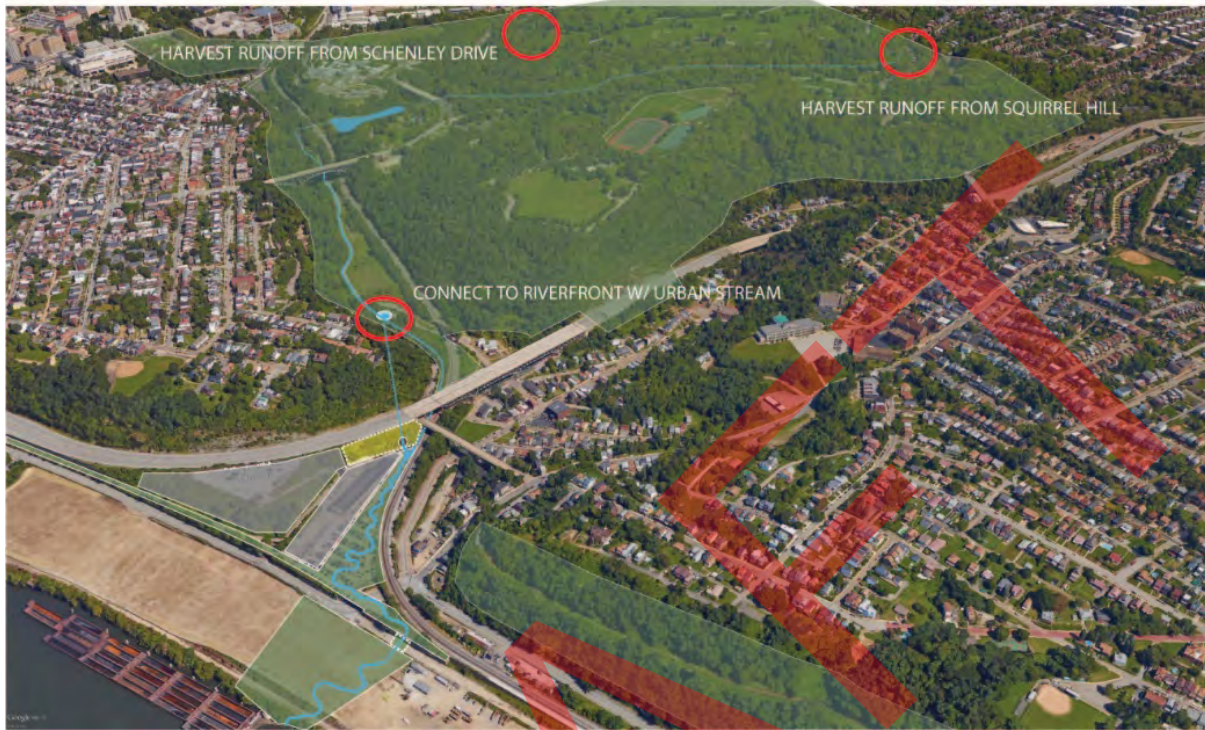
Figure 5-17: Panther Hollow Stream Conveyance Pathway
