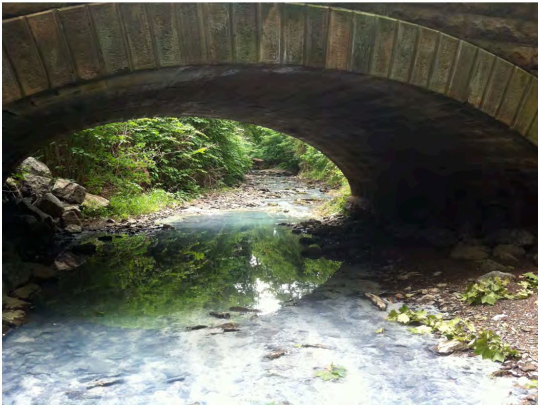
PF57 – Heavy aluminum precipitate covers Piney Fork's substrate at the Stewart Rd bridge crossing at about ½ mile downstream of the Sebolt Rd discharge into Piney Fork.
