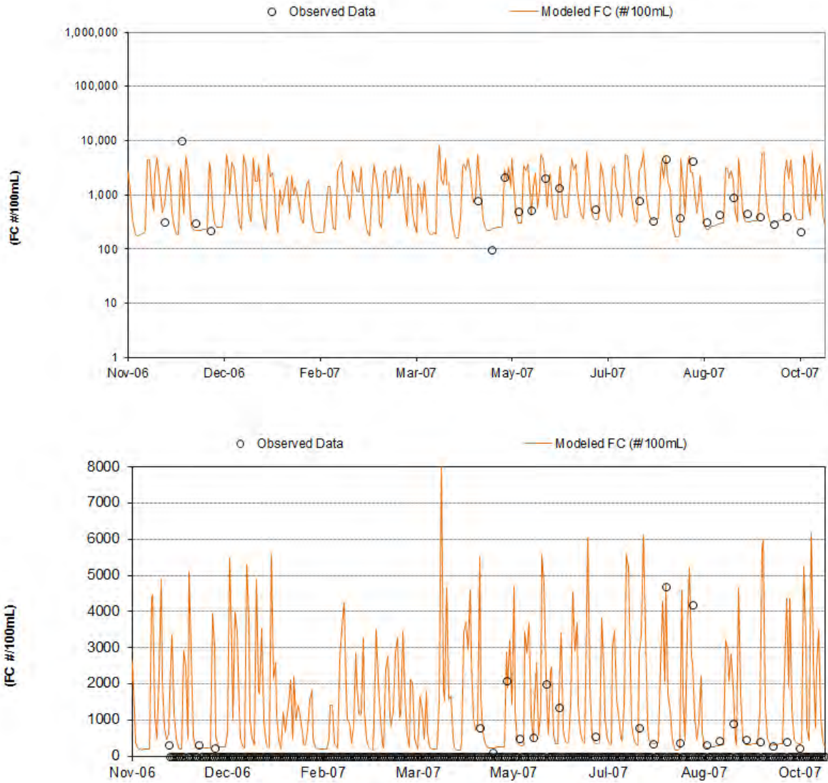
Figure E-7. Bacteria (fecal coliform; CFU/100 mL) calibration at station 7 vs. SWS 7.
