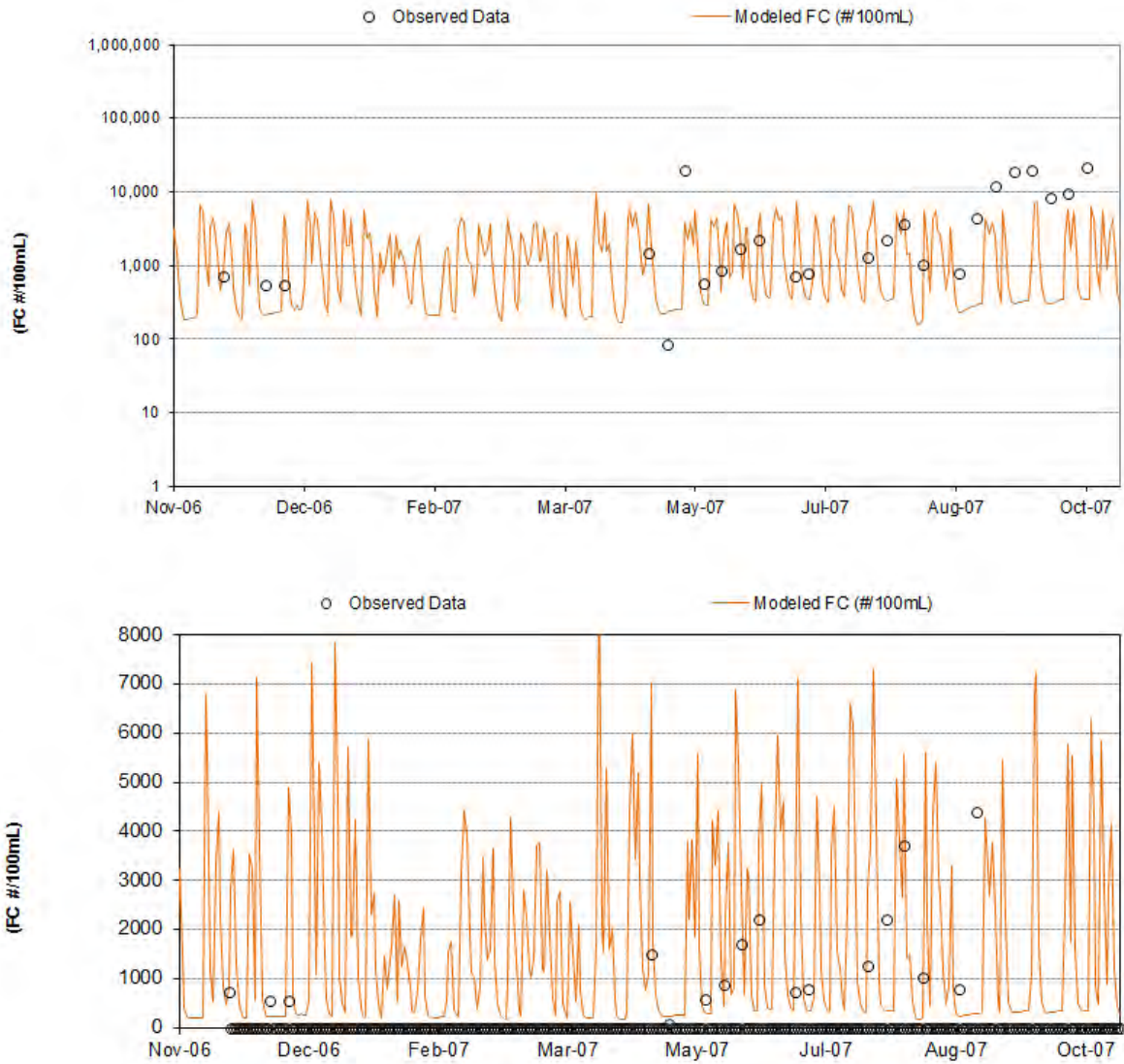
Figure E-1. Bacteria (fecal coliform; CFU/100 mL) calibration at station 1 vs. SWS 2.
