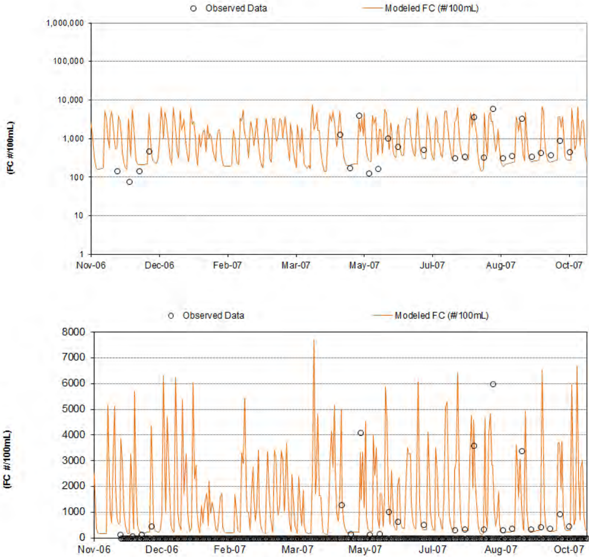
Figure E-9. Bacteria (fecal coliform; CFU/100 mL) calibration at station 9 vs. SWS 13.
