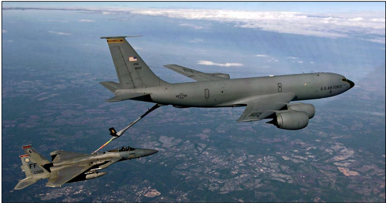
Figure 1.25: an F-15 Eagle fighter jet receives fuel from a KC-135 Stratotanker assigned to the Pennsylvania Air National Guard's 171st Air Refueling Wing over Washington, D.C. U.S. Air Force photo by Staff Sgt. Samuel Rogers, courtesy of 171 st ANG website.
