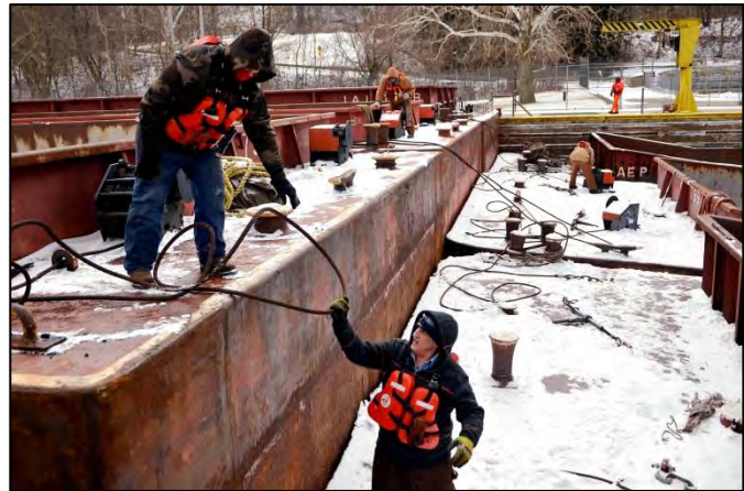
Figure 1.28: Workers lash a tow of barges together after locking through at Montgomery Dam on the bitter cold morning of January 24, 2014. Photo courtesy of the Beaver County Times.
