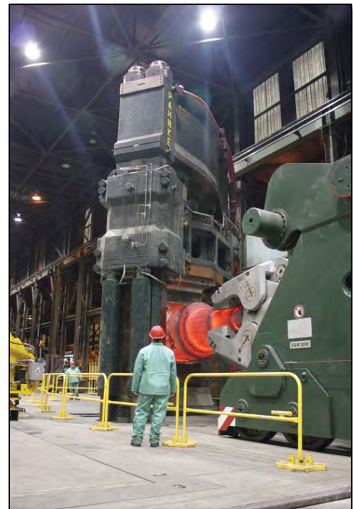
Figure 1.33: Union Electric Steel's 5000-ton hydraulic forge press at its Harmon Creek Plant near Burgettstown. Photo courtesy of UES website.
