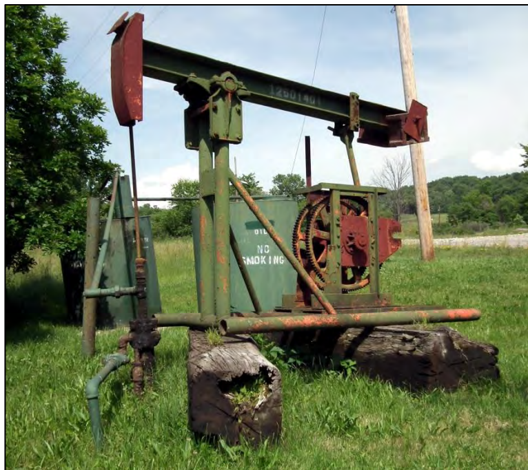
Figure 3.22: One of several pump jacks in the Bonnymeade vicinity of Smith Township. Widely used throughout the U.S. to extract shallow reserves of gas and oil, basic pump jack design has changed little since 1859. Some rural Pennsylvania pump jacks, or “gas donkeys,” have been on the job for one hundred years or more. 6/18/2014.
