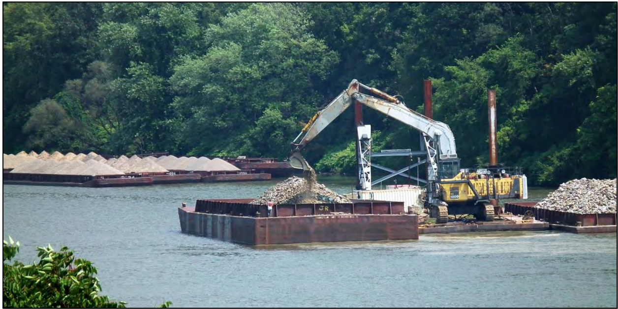
Figure 5.24: An excavator between two barges dredges for gravel on the Montgomery Pool of the Ohio River, 8/5/2014. Note the crewman standing at the corner of the left barge.
