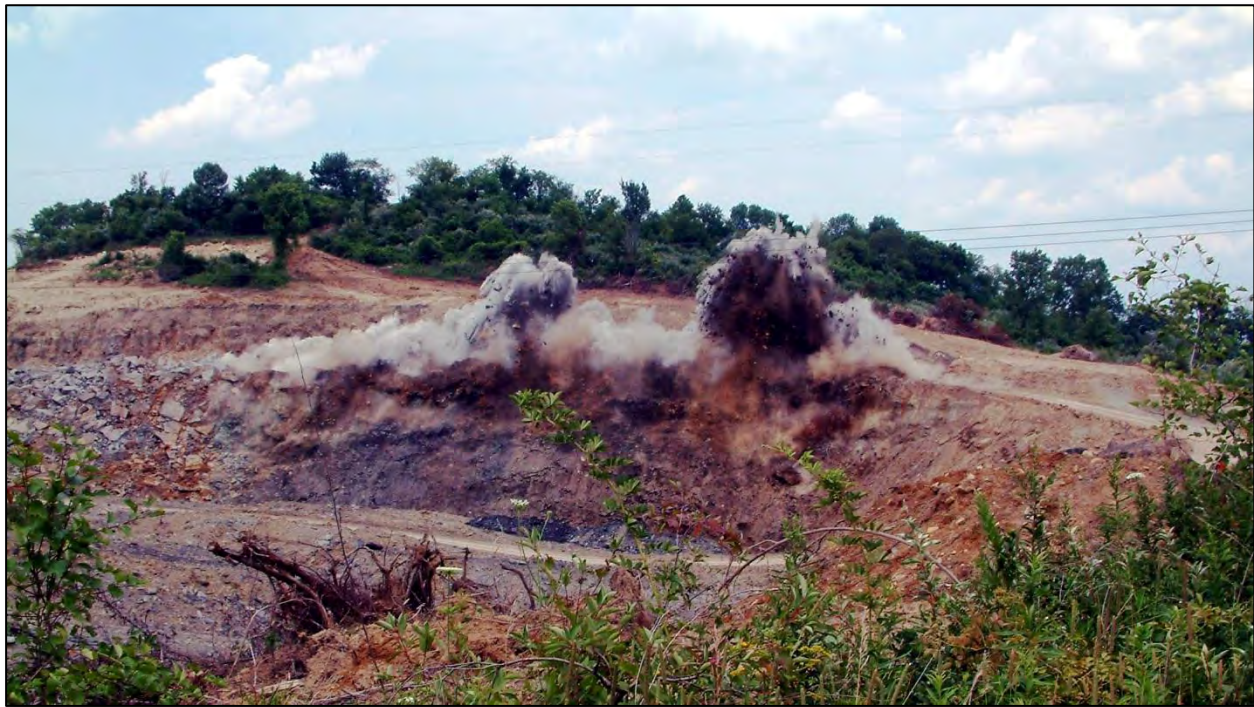
Figure 3.6: Overburden is blasted away to expose the Pittsburgh Coal Seam for re-mining near Burgettstown in the 70c Pittsburgh Low Plateau Ecoregion, 7/17/2007.
