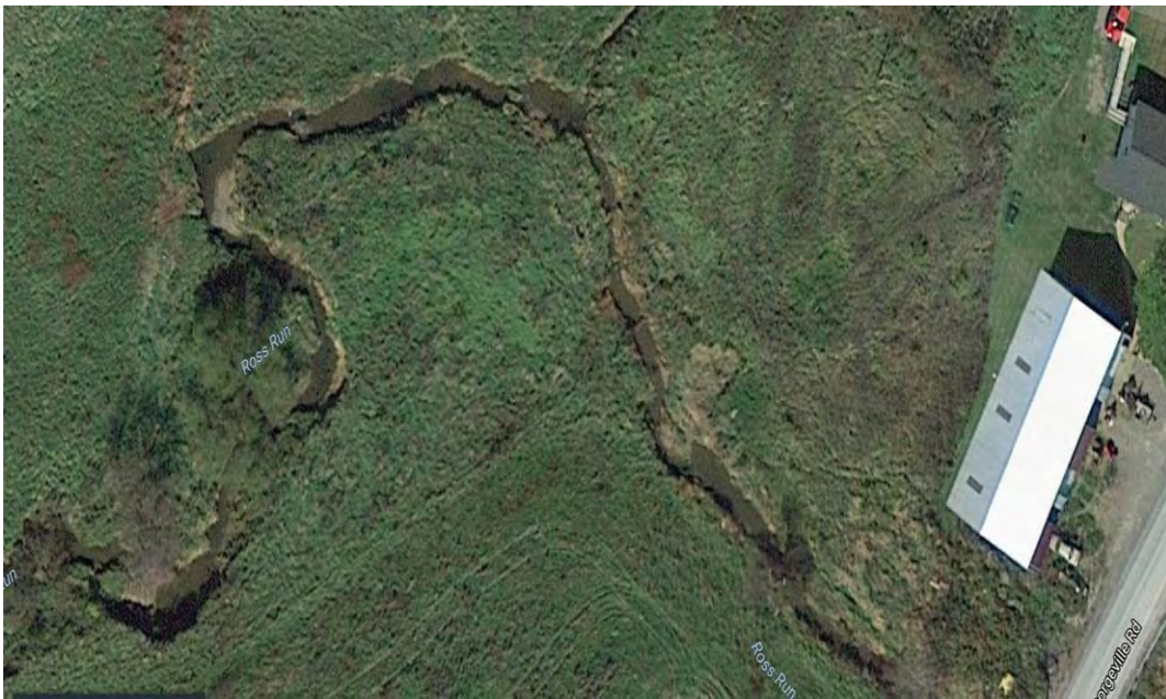
Figure 31. Unconsolidated banks cause frequent and meandering stream bed
