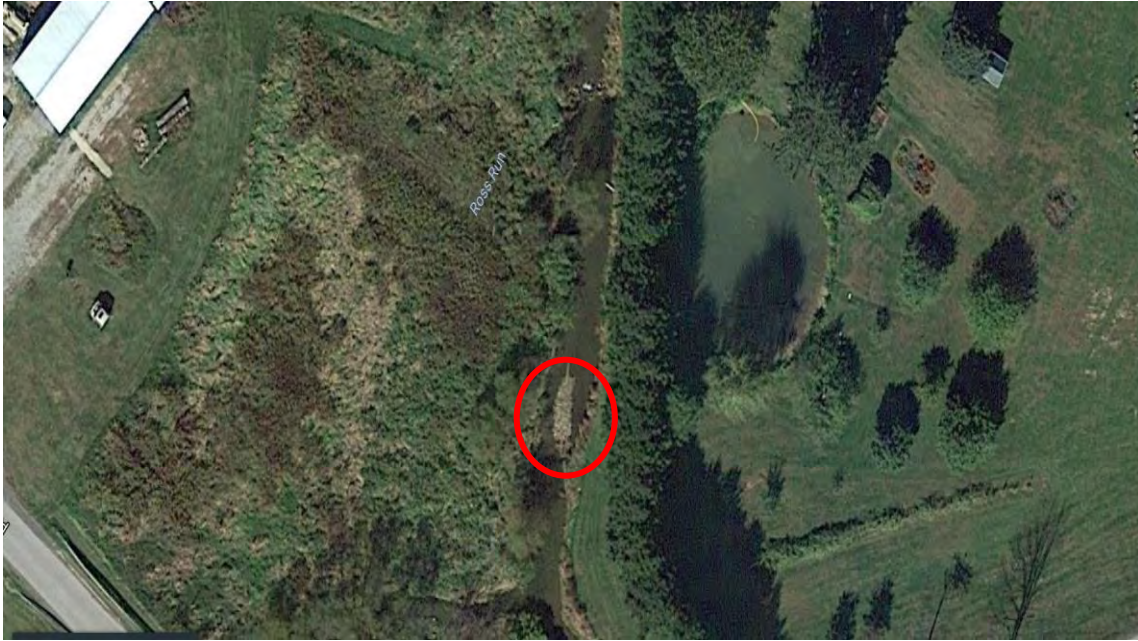
Figure 28. Silt islands forming from upstream loading
