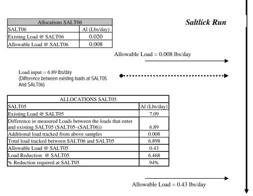
The allowable aluminum load tracked from SALT06 was 0.008 lbs/day. The existing load at SALT06 was subtracted from the existing load at SALT05 to show the actual measured increase of aluminum load that has entered the stream between these upstream sites and SALT05 (6.89).
