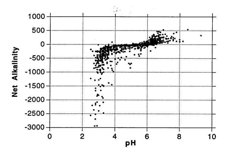
Figure 1. Net Alkalinity vs. pH. Taken from Figure 1.2 Graph C, pages 1-5, of Coal Mine Drainage Prediction and Pollution Prevention in Pennsylvania
