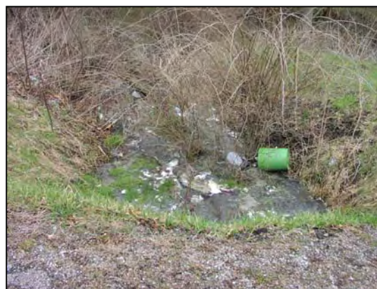
Raw sewage discharging from a malfunctioning on-lot system at Lower Whyel above Yukon in the lower watershed (Source: WPC 2002)
