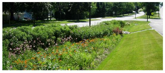
Vegetated swales can be incorporated into a variety of landscapes. Above is an example of a vegetated swale to perform on-site stormwater management and improve aesthetics.
