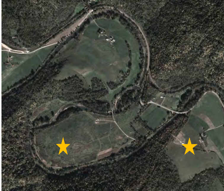
Figure 125. In the Pea Vine Creek subwatershed, AMD from reclaimed strip mine lands on the east and west sides of Dover Ridge Road (York Township Road 729) has been observed entering Captina Creek, but water quality monitoring indicates that it does not impair water chemistry, and dilutes to undetectable levels further downstream (OEPA 2010). Map source: “Dover Ridge AMD.” 39°53’08.38” N and 80°52’40.28” W. Google Earth. October 7, 2011. December 27, 2012.
