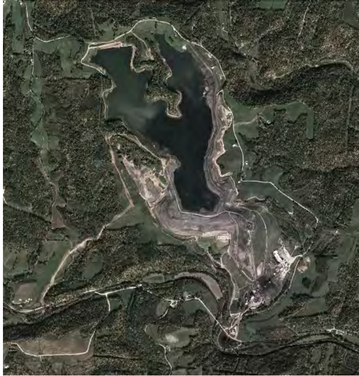
Figure 117. The OVCC Powhatan No. 6 mine and slurry impoundment facility near Alledonia, Ohio. The impoundment discharges into an artificially constructed outfall drainage to Captina Creek west of the Powhatan #6 mine. Although NPDES permit violations have occurred in the past, the Powhatan #6 mine remains below acceptable parameters for discharging metals and currently has no defined limits on discharging total dissolved solids (Wood-Pugh, personal communication, 2011). Photo source: "OVCC Slurry Impoundment." 39°55'08.23" N and 80°59'32.11"W. Google Earth. October 27, 2011. October 22, 2012.
