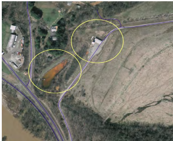
Figure 128. A dosing silo and settling ponds, located near the intersection of Cove and Lysein Roads just west of Powhatan Point (Cat Run subwatershed), treat acidic water pumped out of abandoned mine shafts with alkaline material before it can enter Captina Creek. This site is the former location of Bellaire Corporation's Powhatan No. 2 coal mine. Additional remediation is planned by North American Coal, the current owner of the site. Photo source: Google Earth.
