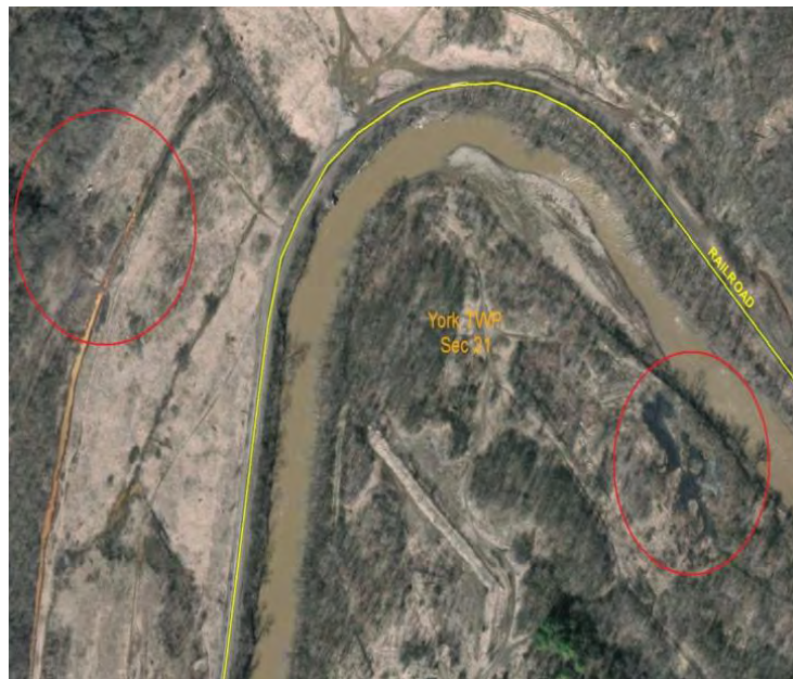
Figure 126. Remnants of two small gob piles exist in Section 21 of York Township (Pea Vine Creek subwatershed), originally occupied by Bellaire Corporation Powhatan No. 5 coal mine. This site was also the former location of a limestone gravel pit. AMD draining from the site does not impair water chemistry, and dilutes to undetectable levels further downstream (OEPA 2010).
