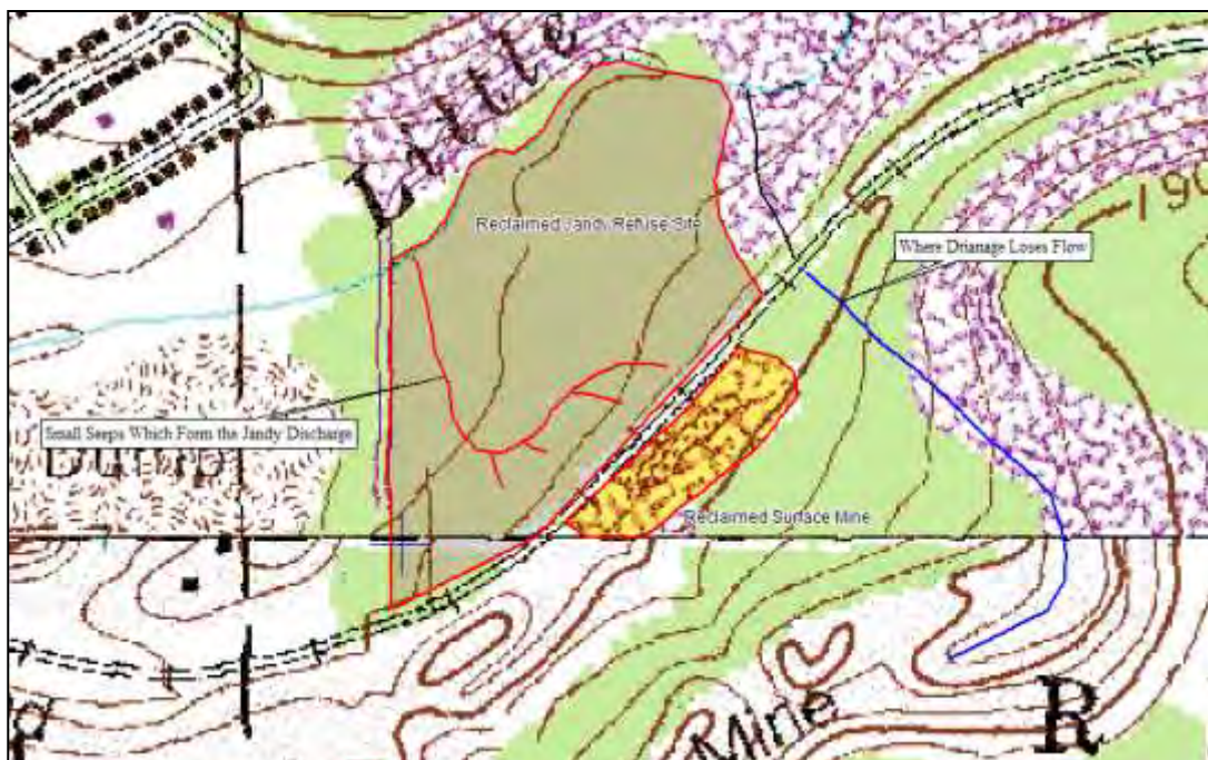
Figure 18. Drainage pattern of Jandy Discharge
