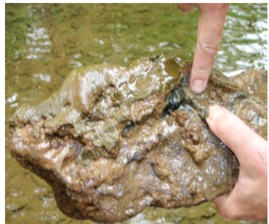
Figure 15 Mineral deposits on substrates create a concrete-like structure, typical in mineral rich mine water.
