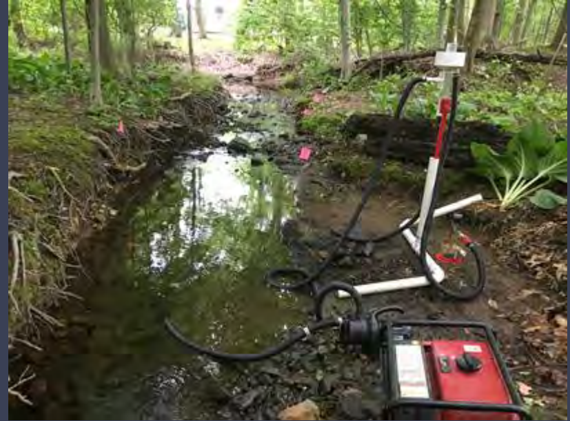
AKRF in-situ measurement of bank erodibility
